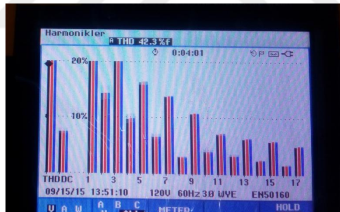
Figure 4.25 THD voltage measurement using FLUKE 435 Power Analyzer.
