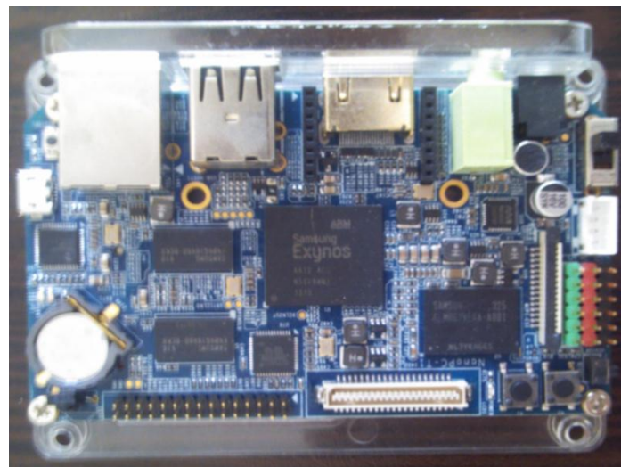
Figure 3.22 Single board computer
