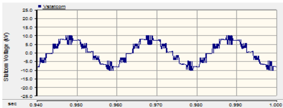
Figure 5.37 Statcom voltage before arm inductor in inductive mode using phase-shifted PWM balancing
