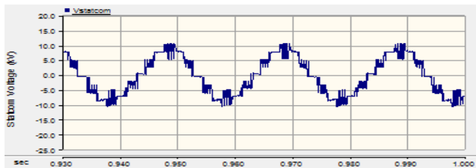
Figure 5.34 Statcom voltage before arm inductor in capacitive mode range using phase-shifted PWM balancing
