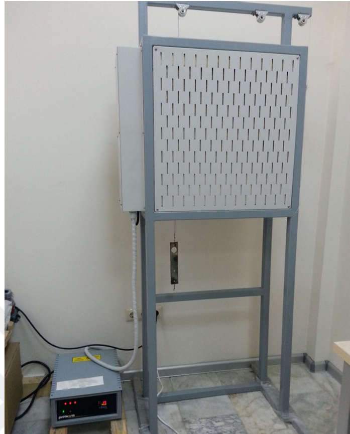
Figure 2.7. Vertical Drying Furnaces
