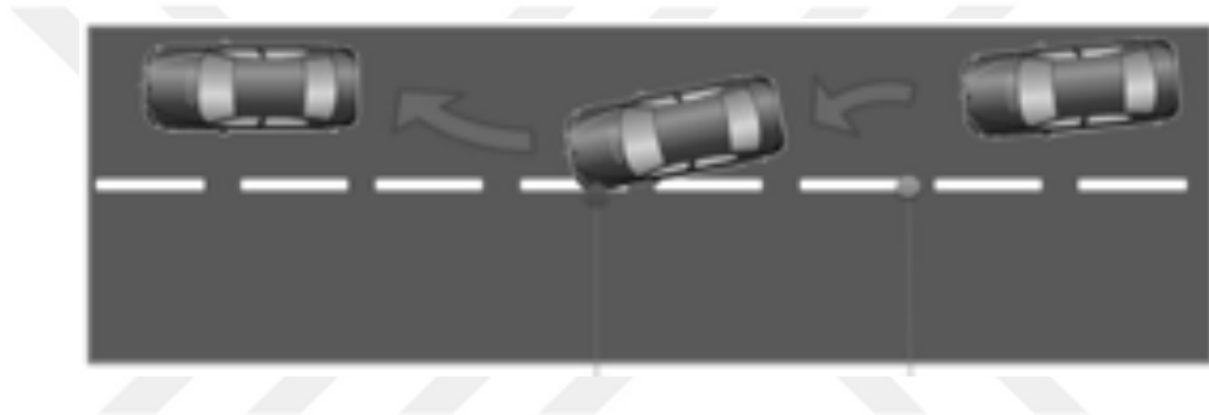
Figure 4.60 LKAS controls systems [133].
