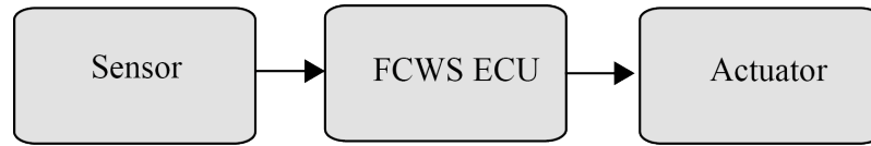
Figure 4.32 FCWS block system.
