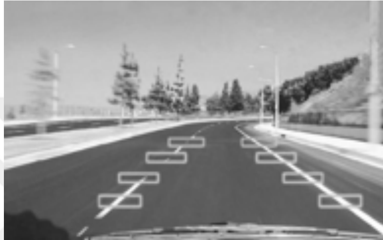
Figure 4.58 Detection system for lane [136].
