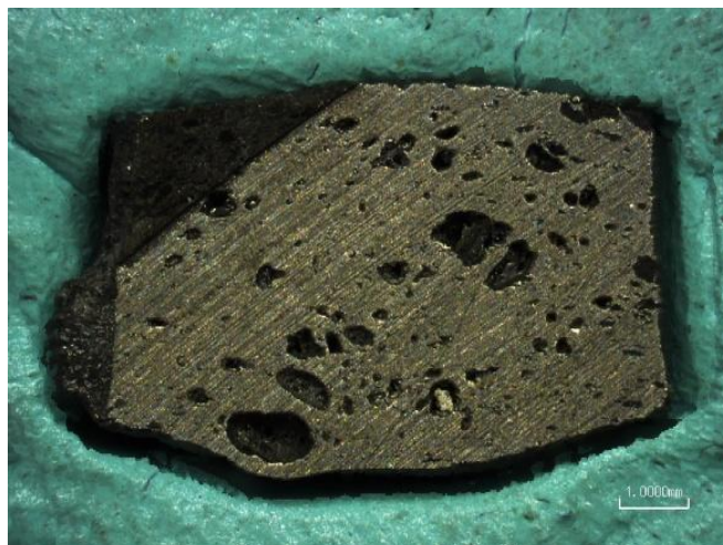
Figure 3.54 Image of the sectioned W**HAS prepared from W** powder, sintered at 1500 °C for 1 h.
