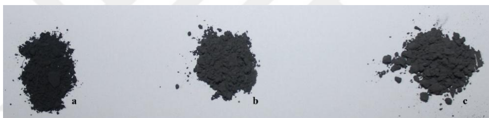
Figure 3.56 Colors of the employed tungsten powders (a:W** powder, b:W* powder, c:W powder).
