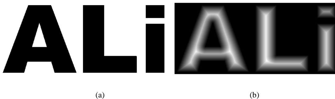
Figure 3.10 Application of distance transformation (a) binary image as an input (b) distance transformation of the image
