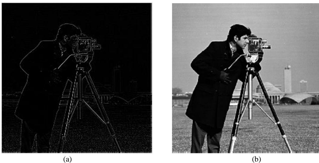
Figure 3.18 (a) High pass filter applied cameraman image, (b) sharpened cameraman image with k = 1
