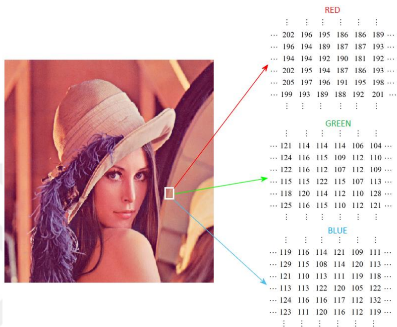
Figure 3.5 Lena image and three intensity values of the determined area. Each color intensity value storage requires 8-bit and totally 24-bit
