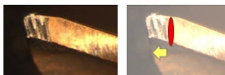
Figure 1.10 The different wear types on the carbide drills [24].
