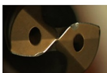
Chipping on main edge
