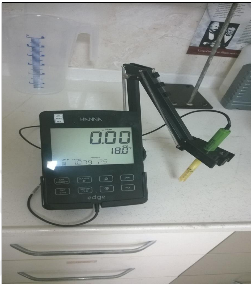
Figure 4.11 The pH meter.
