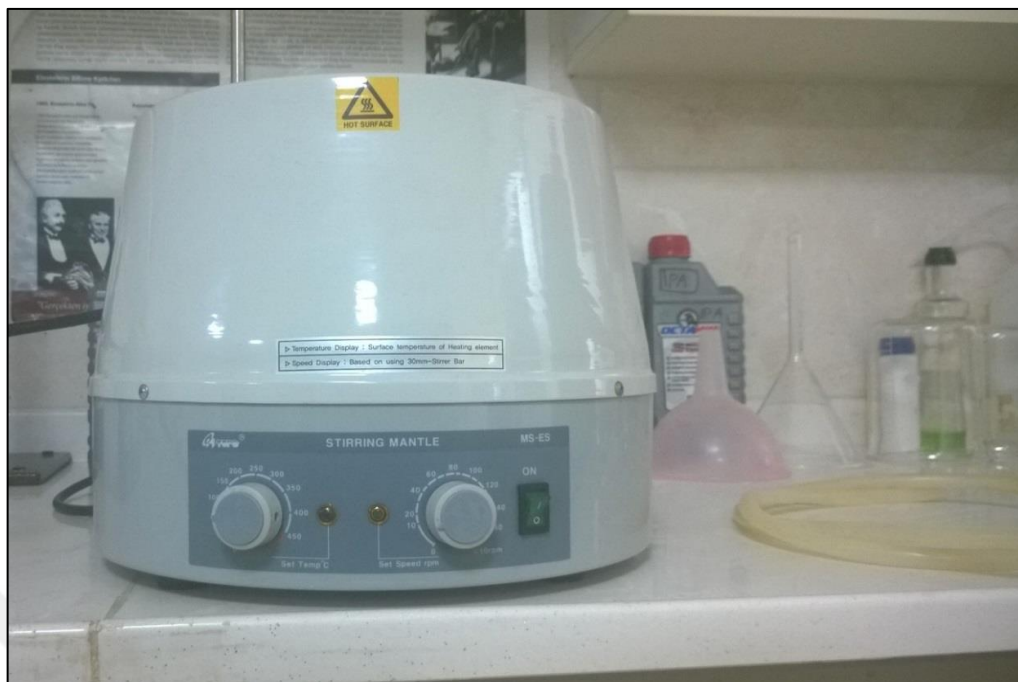
Figure 4.10 The stirring mantle.
