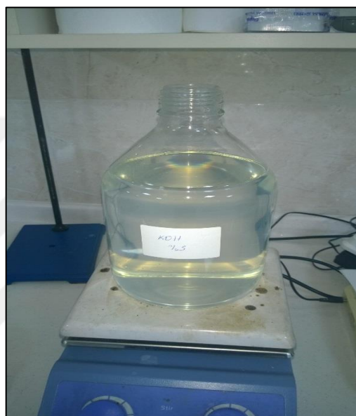
Figure 4.5b Preparing of KOH solution.
