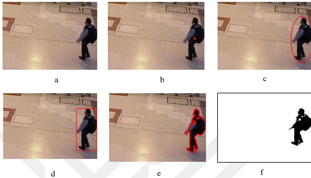
Figure 2.1 (a) cropped image from PETS 2006 dataset [17], object represented by (b) a point, (c) an ellipse, (d) a rectangle, (e) contour and (f) silhouette.
