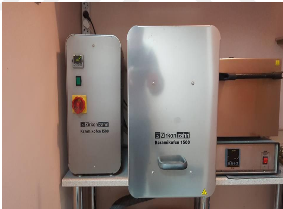
Figure (7) Special oven used for sintering zirconium disks.
