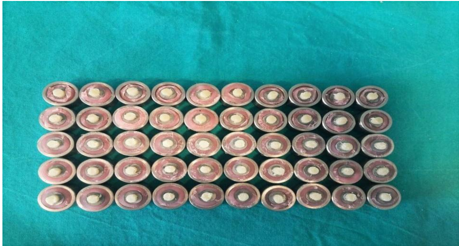
Figure (27) Fixed all Ni-Cr disc in steel mod using acrylic resin
