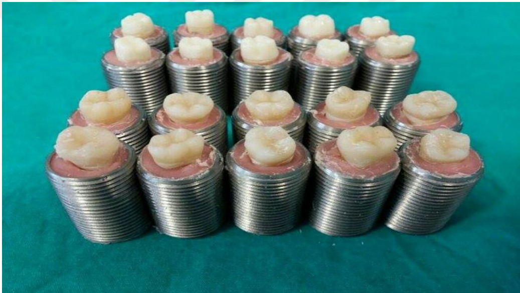
Figure 19: Mounting all spacemen in acrylic resin
