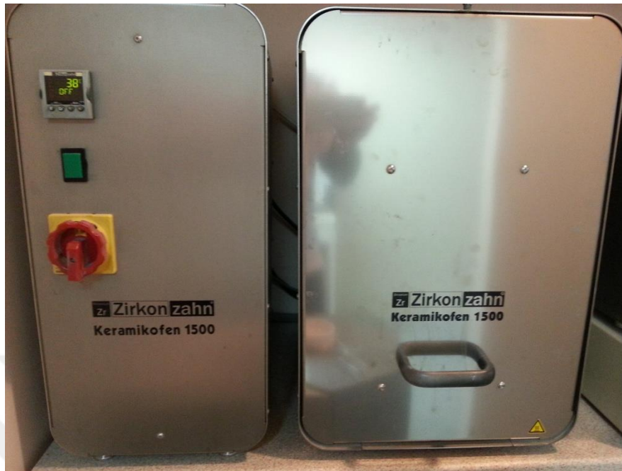
Figure-7: The Furnace Used for Sintering Zirconia Discs
