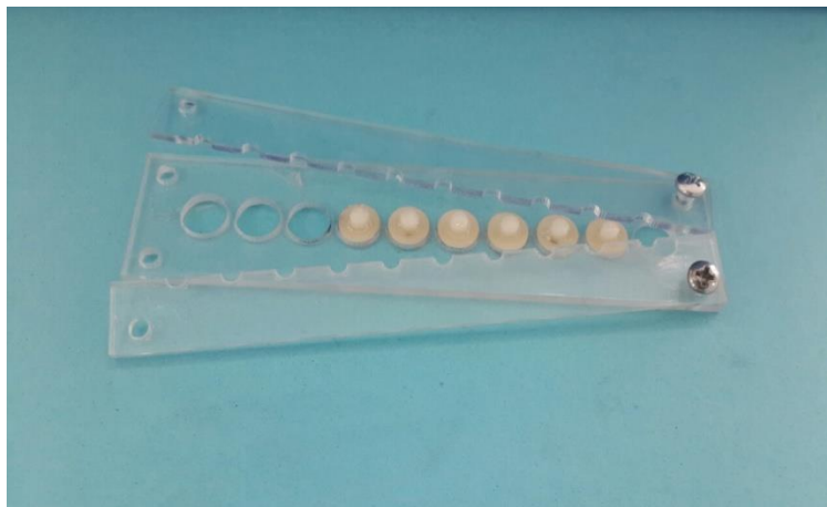
Figure-22: Remove the Plexiglas Mold from Zirconia Specimens
