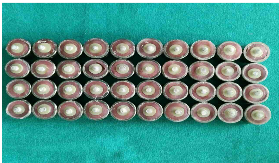
Figur-27: The Zirconia specimens after adhered it by self cure acrylic resin a stainless steel mold.
