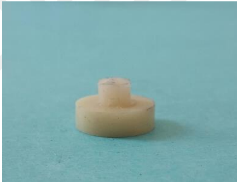
Figure-23: Self-Adhesive Resin Cement after Complete Curing
