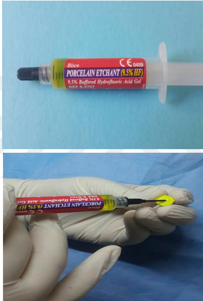
Figure-15: Etching of Zirconia Specimens by Hydrofluoric Acid
