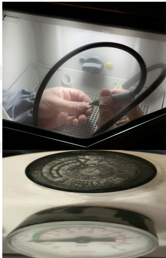
Figure-14: Sandblasting Machine with Pressure 0.2 Mpa
