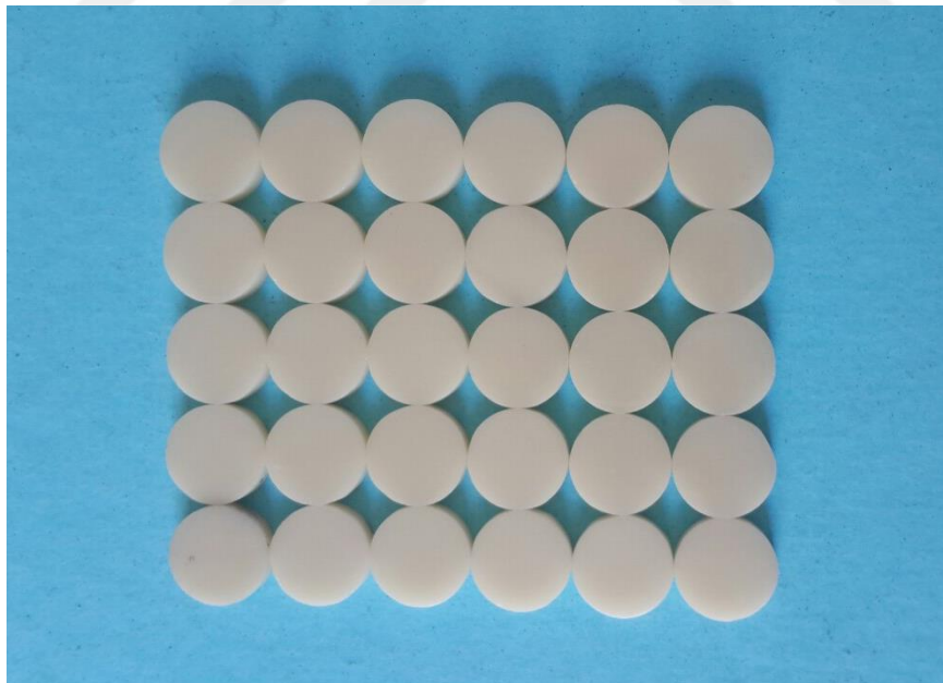
Figure-8: Zirconia Discs after Sintering
