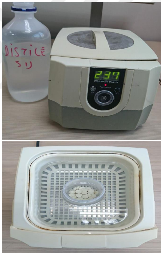
Figure-12: Ultrasonic Cleaning Machine Used with Distilled Water
