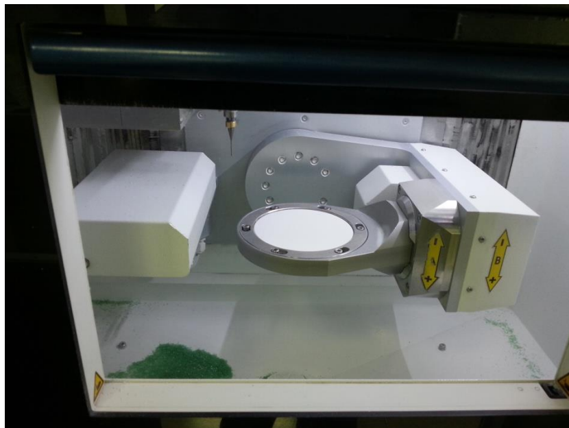
Figure-4: Place the Zirconia Block in the CAD/CAM Machine
