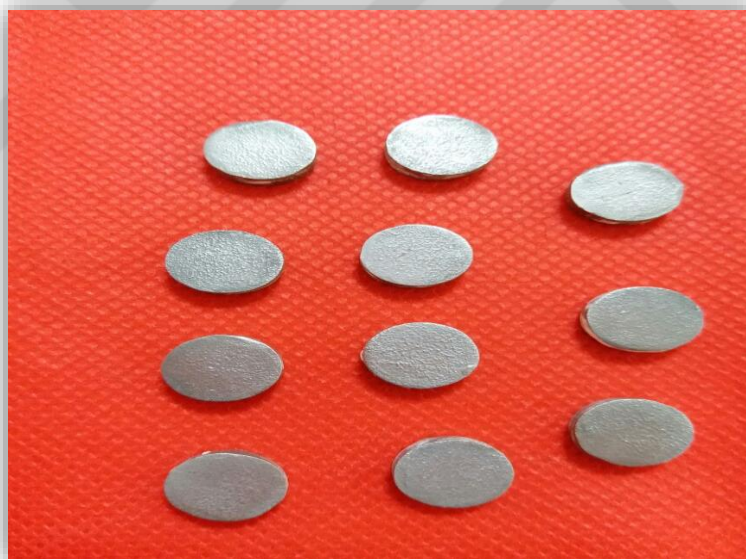
Figure (12) the final shape of metal discs after sandblasting.
