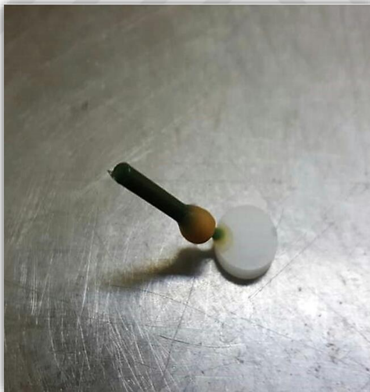
Figure (4) the sprue attached to the wax disk
