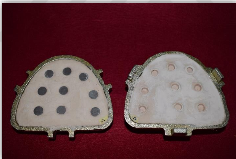
Figure (17) the shape of the specimens after wax melted.
