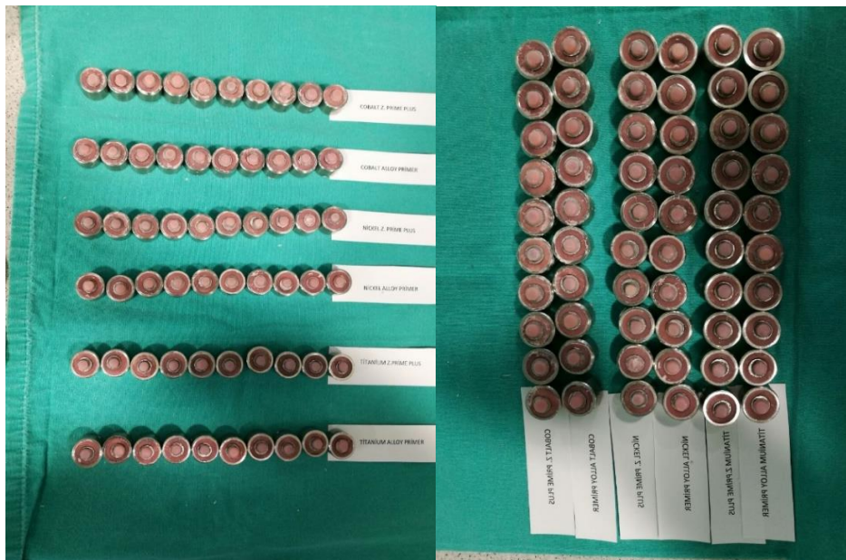
Figure (35), (36) all the 60 samples are ready to measure SBS
