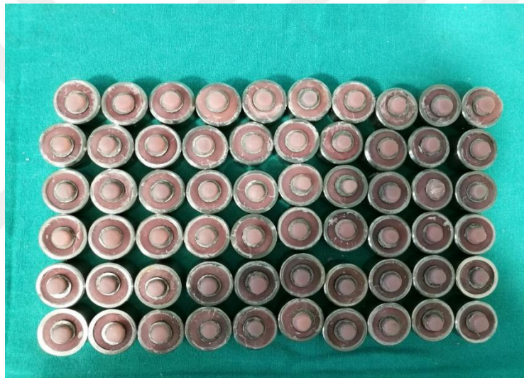
Figure (34) the samples inside the self –cure acrylic resin.
