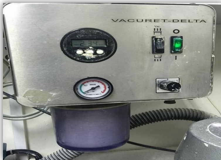
Figure (6) Vacuret-delta machine used to mix phosphate bonded investment material for metal casting.
