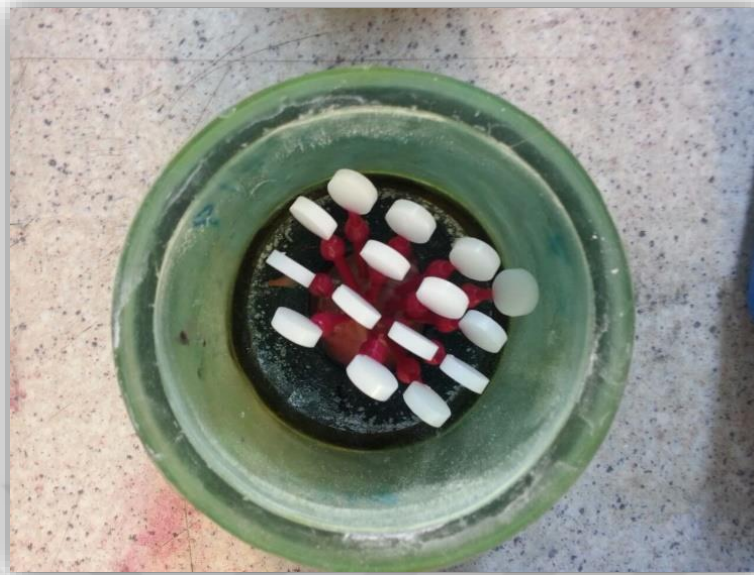
Figure (5) all the attached sprue wax disks connected to crucible former.
