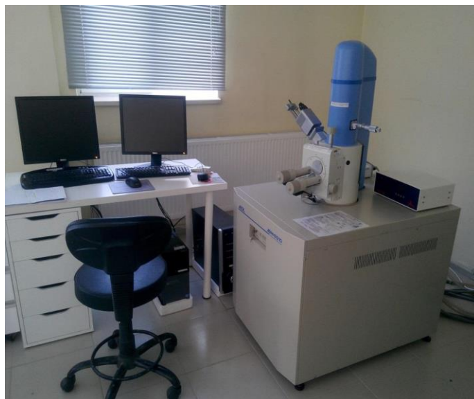
Figure 3.13. The EDX and SEM system we use in our studies (JEOL JSM-6510)
