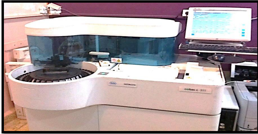
Plate 3.1. Cobas c 311 fully automated biochemistry analyzer
