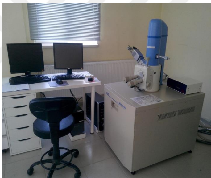
Figure 3.12. The EDX and SEM system we use in our studies (JEOL JSM-6510)
