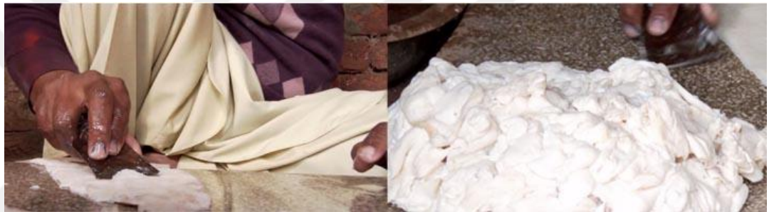
6.7 – Artisan scraping of the skin and collecting a mash of it (IRC, 2015).
