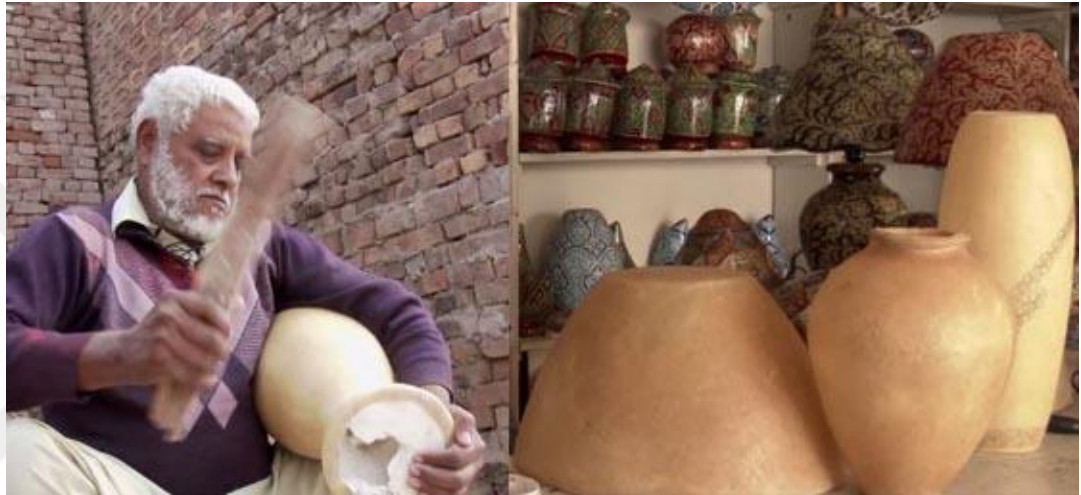
6.9 – Artisan breaking the mold inside the dry camel skin cast to get the forms for making lights (IRC, 2015).
