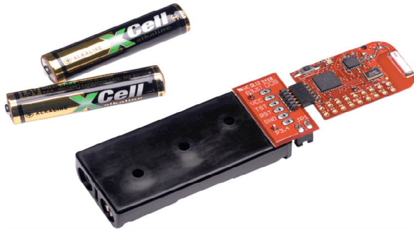
Figure 6.6: eZ430-RF2500 End device Battery Board (Slauu227e, 2009)
