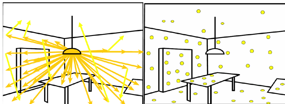
Figure 2.7 The left image shows the casted rays from the light source. The right image shows the photons that are chosen with respect to the interaction points of the casted rays (Bouatouch, 2012)
