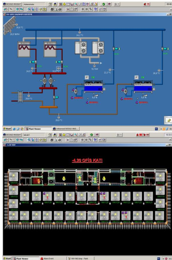
There is an automation system which automatically engages and unmounts all the cooling, electricity and mechanical systems of the whole building. It is aimed not to use energy more than necessary and to operate the systems with full performance with this system (Figure 4.9.).
