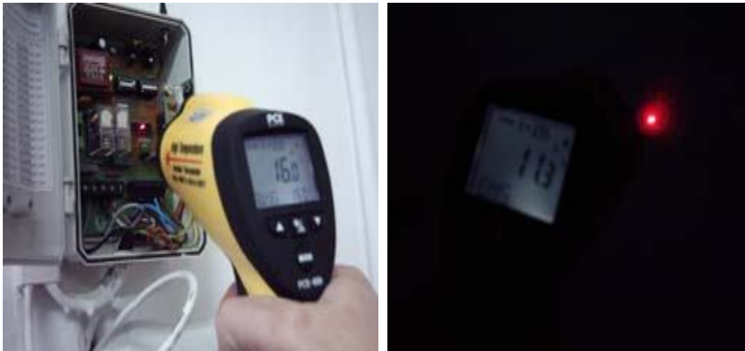
Figure 17. Temperature Measurement With Infrared Thermometers
