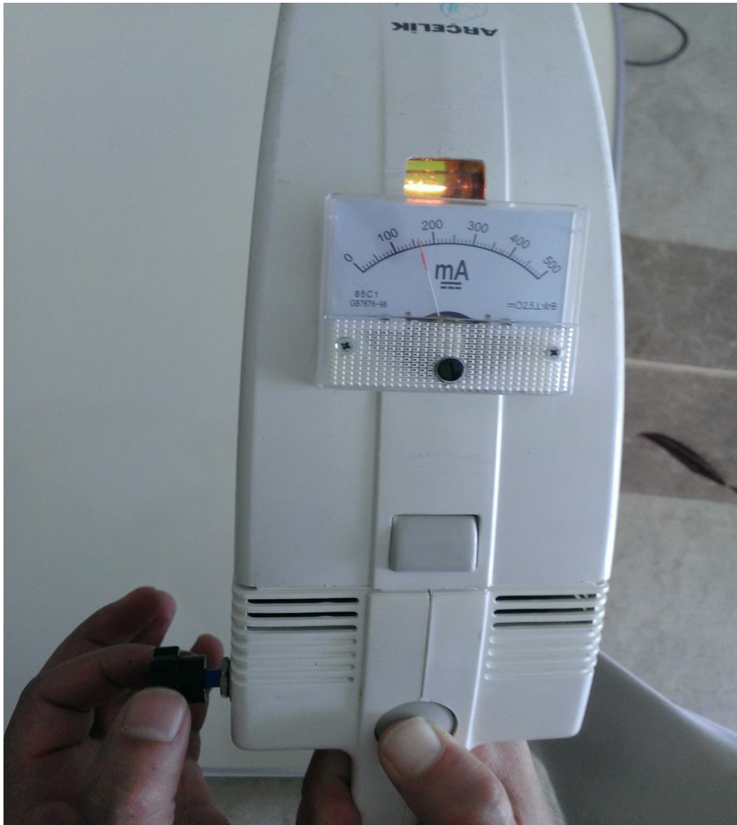
Figure 25. Handmade Optical Pyrometer
