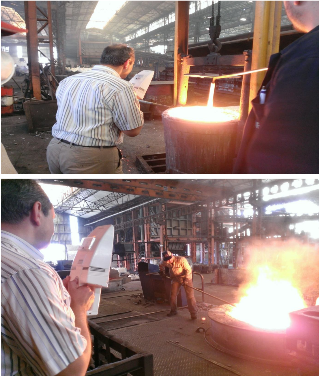
Figure 28. Calibration With Dip-type Thermocouple at "Şafak" Casting Factory
