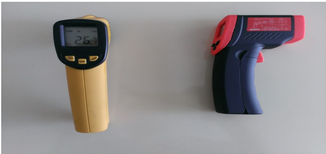
Figure 26. TECMAN TM550 Infrared Thermometer
