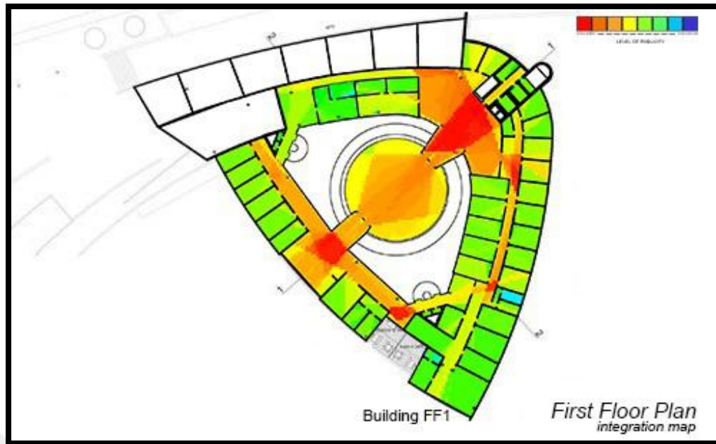
Figure 4.31 Karabük Municipality Service Building Competition, First Prize, Integration map of first floor plan
