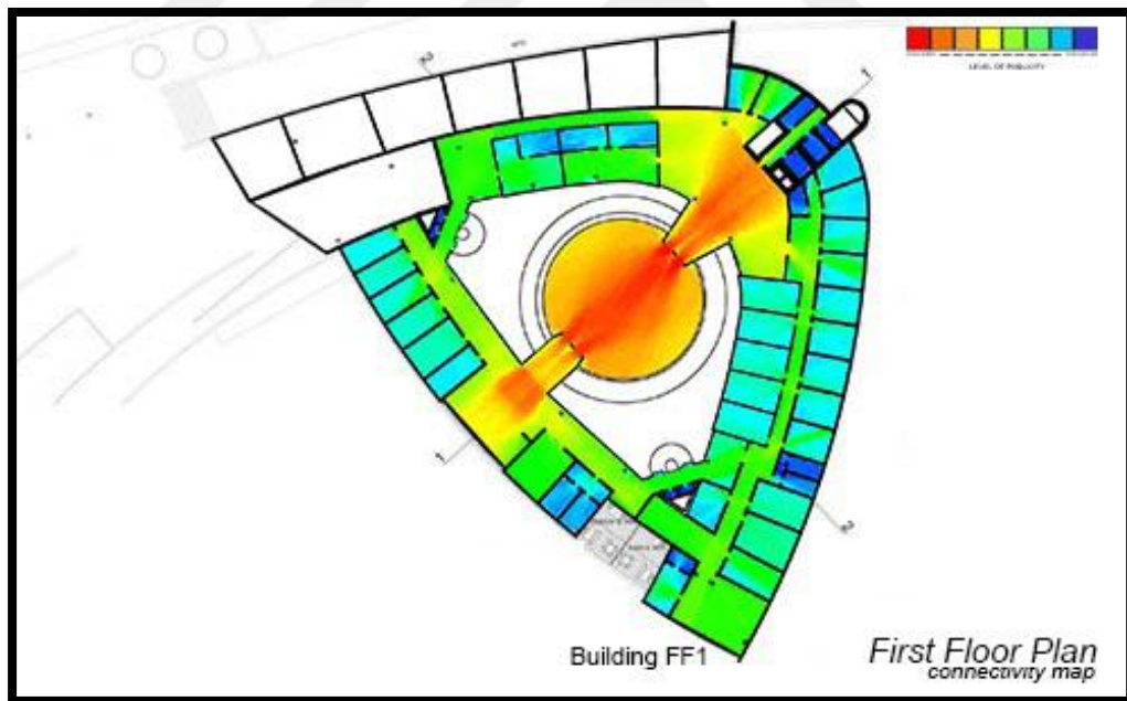
Figure 4.30 Karabük Municipality Service Building Competition, First Prize, Connectivity map of first floor plan
