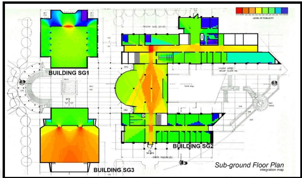
Figure 4.5 Gaziantep Municipality Service Building Competition, First Prize, Integration map of sub-ground floor plan
