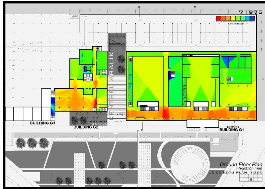
Figure 4.13 Gaziosmanpaşa Municipality Service Building Competition, First Prize, Integration map of ground floor plan
