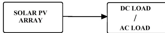
Figure 1.4 Block diagram of Direct Coupled PV Solar System
