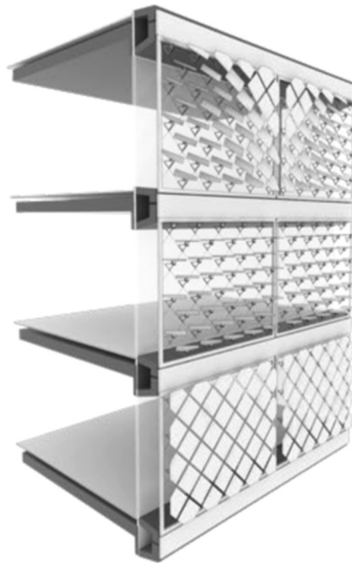
Figure 8. Orientation parameter drives each of the PV panels. (Nagy et al., 2016)
