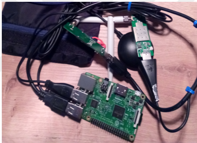
Figure 4.4: Raspberry Pi 3 with External Wireless Adapters and a GPS module
