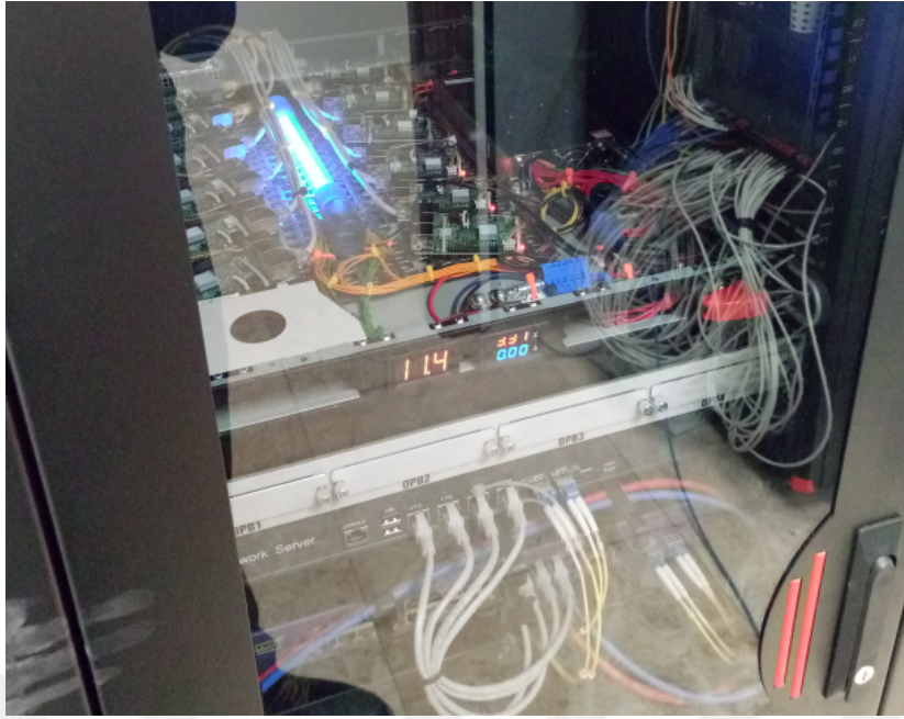
Figure 4.3: 12x Raspberry Pi 2/3 Traffic Generator Nodes
