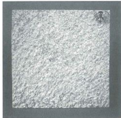
The same texture seen under straight-on or diffused light. Note the lack of shadow from the pushpin.
