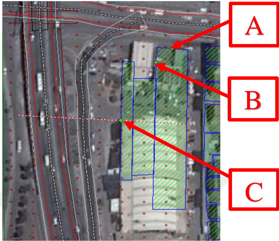
Figure 33 Facade Noise Receiver Points
