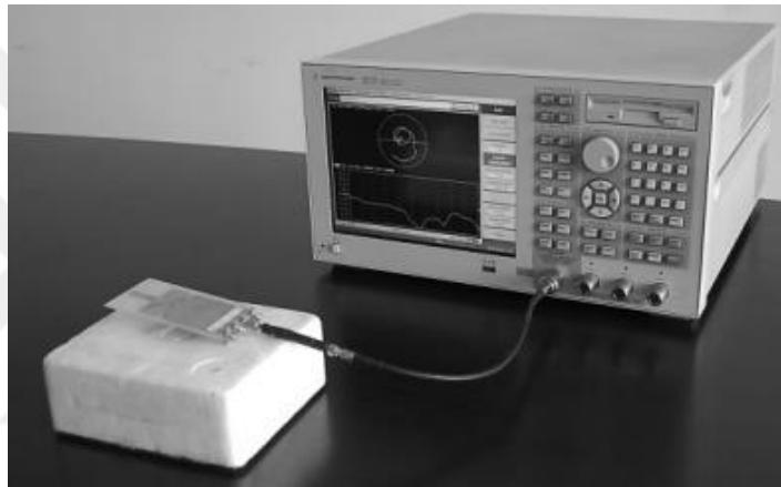
Figure 2.16. Antenna testing setup on a vector network analyzer
