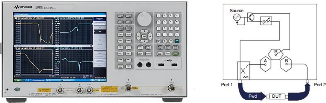
Figure 2.15. Sample vector network analyzer with its simplified schematics
