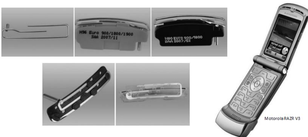
Figure 1.25. Various practical implementations of folded monopole antennas (Zhang, 2017)
