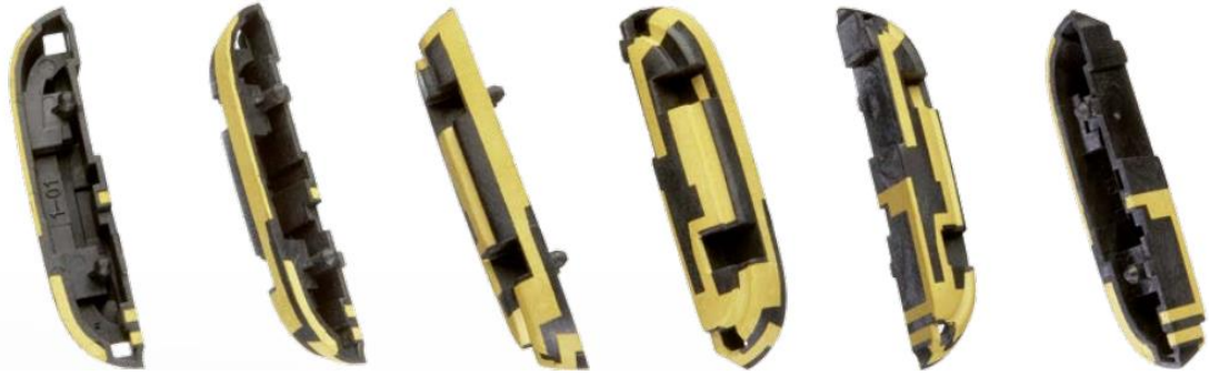
Figure 2.14. Three-dimensional structuring on carrier plastic by LDS (LKPF,2017)
