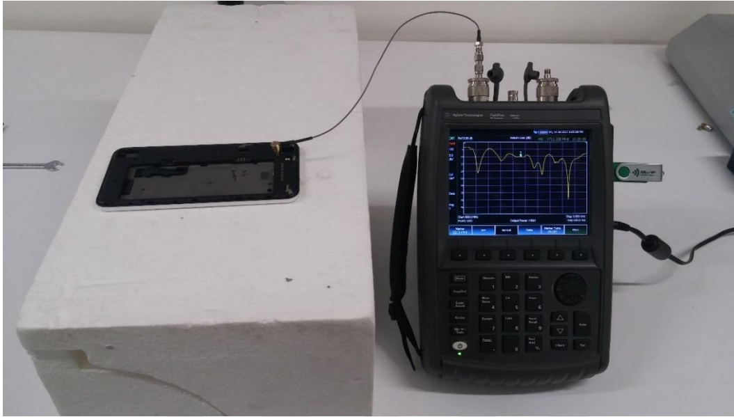
Figure 3.16. Physical setup for measurement of Return loss (dB) of diversity antenna
