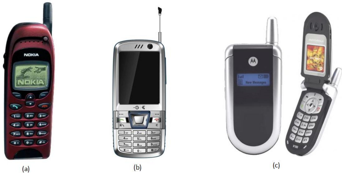
Figure 1.9. Mobile phones with external antennas (a) Nokia 6150 (Stubby Antenna), (b) Telstra explorer 165 (Retractable Antenna), (c) Motorola V180 (Stubby Antenna)
