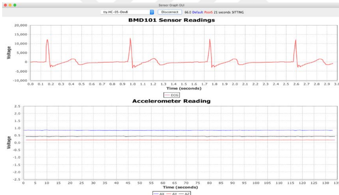
Figure 5.14. Heart Signal and Accelerometer Signal of Sitting Person
