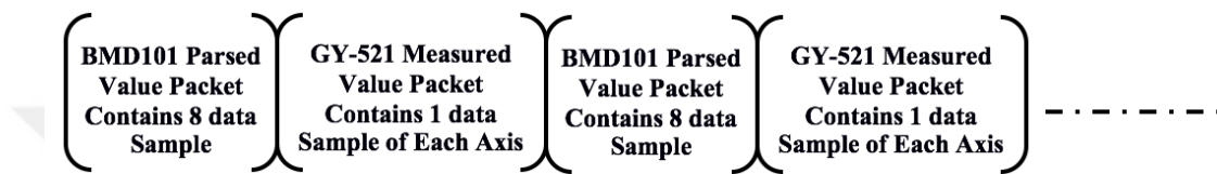
Figure 5.13. Serial Data Packet of ECG Device
