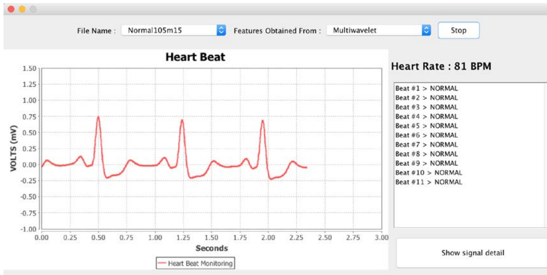
Figure 4.17. Simulating Signal and Labelling the Beats
