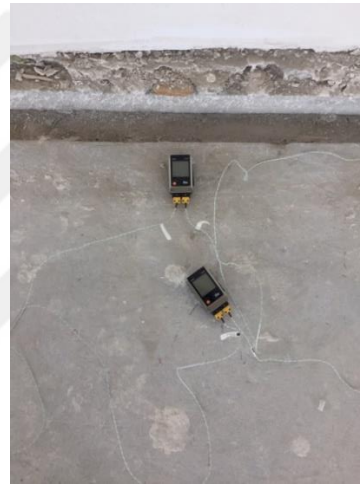
Figure 21. Placement of temperature sensors (office view)
