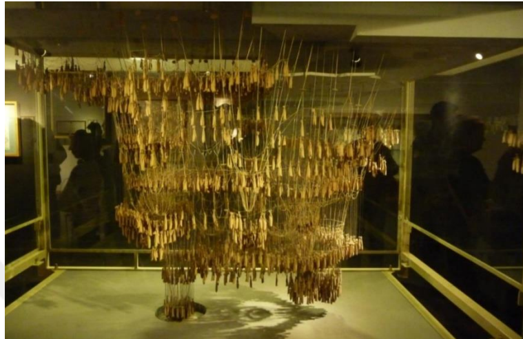
Figure 3.4. Gaudi's hanging chain model reproduction (Asmaljee, 2014).
