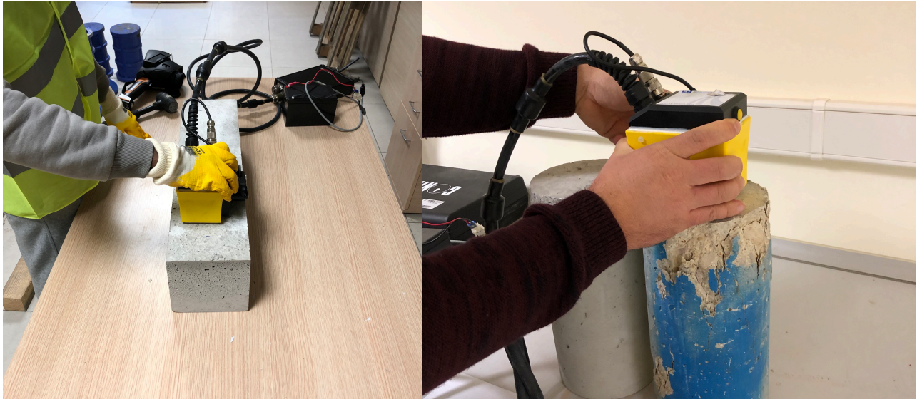
FIG 4.6. Taking GPR Reading
