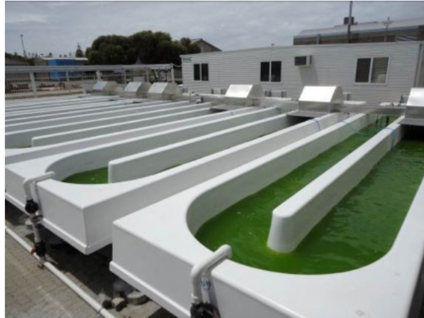
Figure 3.1 Open System Microalgae Cultivation Pond (“Kültür Sistemleri-Algler,” n.d.)
