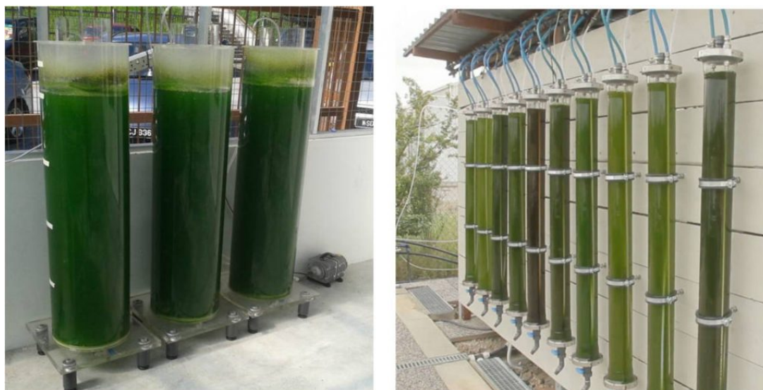
Figure 3.3 Vertical (Bubble) Column Photobioreactor (“Kültür Sistemleri-Algler,” n.d.)
