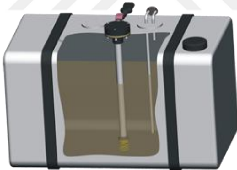
Figure 3-20 Installation prototype of the fuel level sensor into the fuel tank
