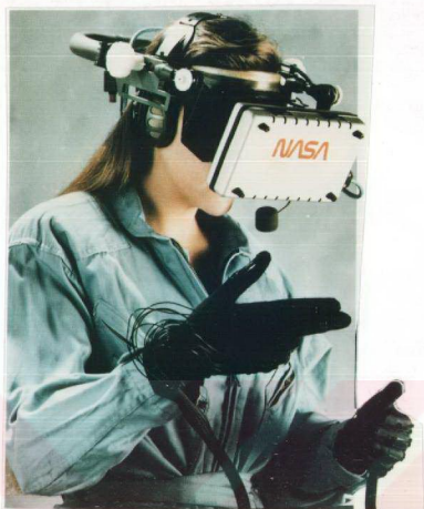
Figure 12. Head-mount display device with sensory gloves (Brill, 1992)
