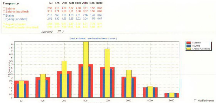
Figure 27. Estimated reverberation times of quick estimate for unoccupied hall.
