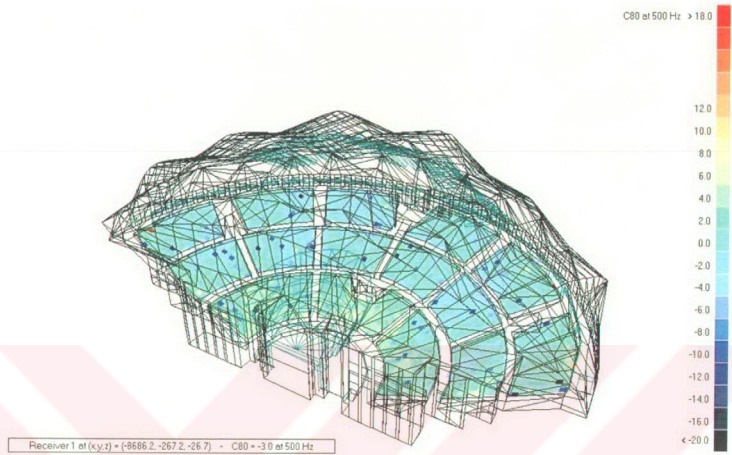
Figure 102. Clarity distribution map for 500 Hz and for the renovated hall.
