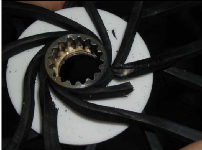
Figure 4.2. Flex pack failure (Moore et. al, 2004, p. 15)
