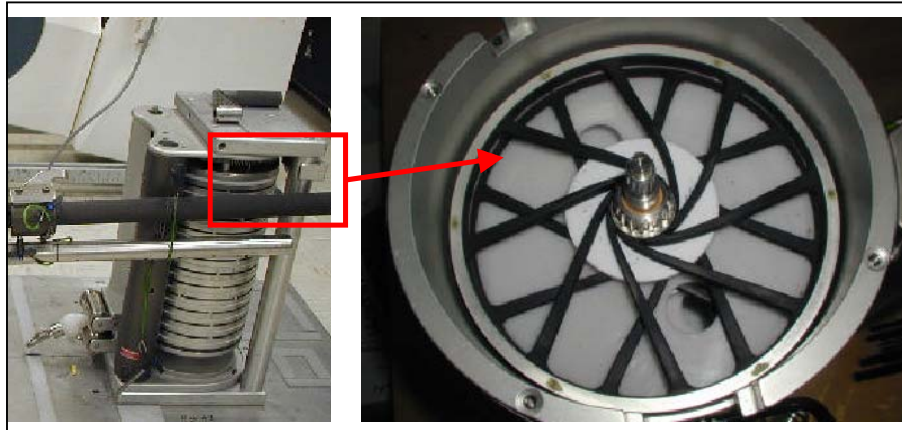
Figure 3.5. Top view of a flex pack in the iRED (Moore et. al, 2004, p.3)
