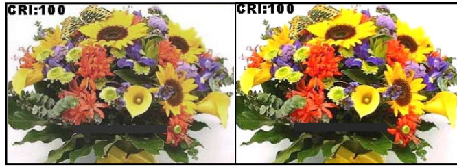
Figure 2.2. Effects of Two Separate Lamps Having Identical CRI Values, but Different Chromaticity Coordinates. http://www.donsbulbs.com/bulbs/g/glossary/cri.example7.jpg
