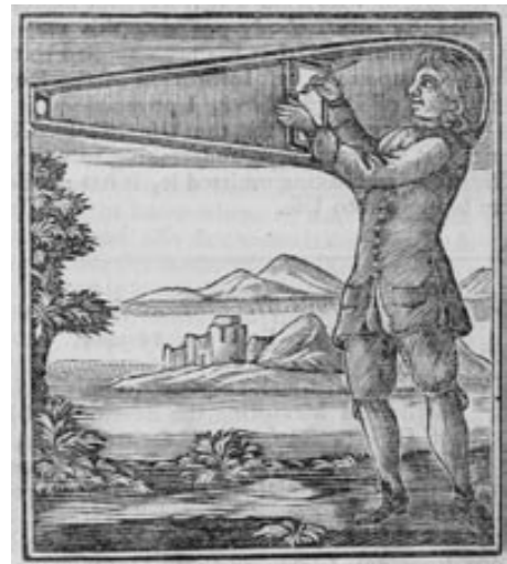
Figure 3.7. Hooke's portable camera, 1694 (Burns, 1999).
