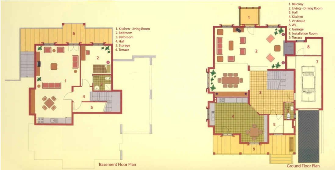
Figure 3.6. Basement and ground floor plan of semi-detached villas (Angora Evleri Advertisement Booklet)
