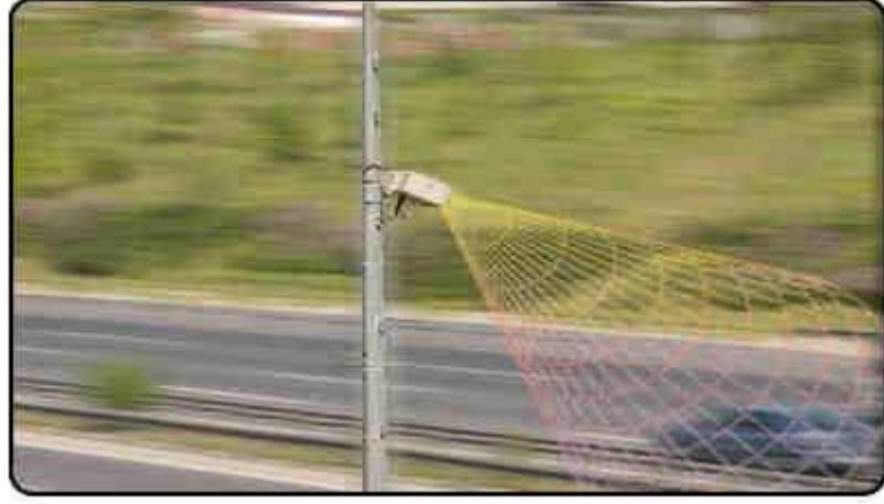
Şekil 2.5 : Yol kesmeyen (non-invasive) sensör (Url-5)
