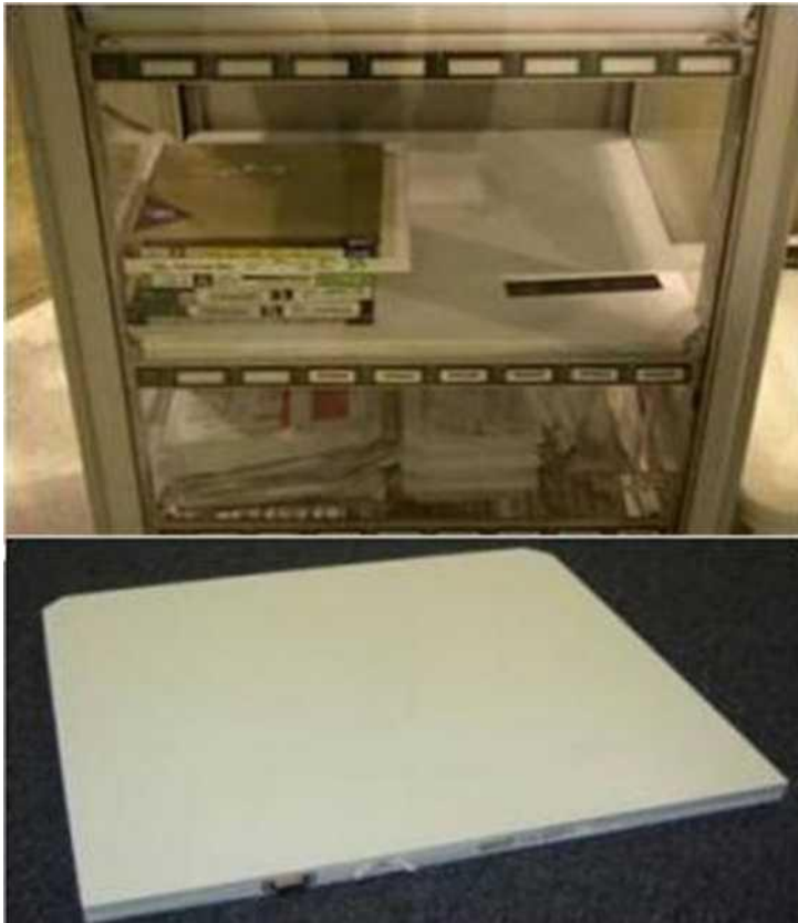
Figure 2.4 : RFID Smart shelf with NF antennas (Venture Research Inc., 2013)
