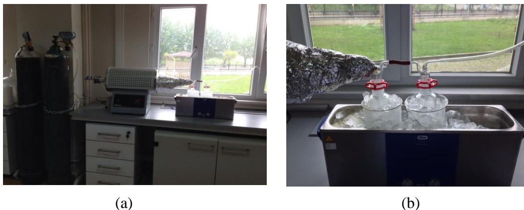
Figure 5.1: (a) Experimental setup for pyrolysis of olive pomace (b) sequential condensers for trapping pyrolysis vapors
