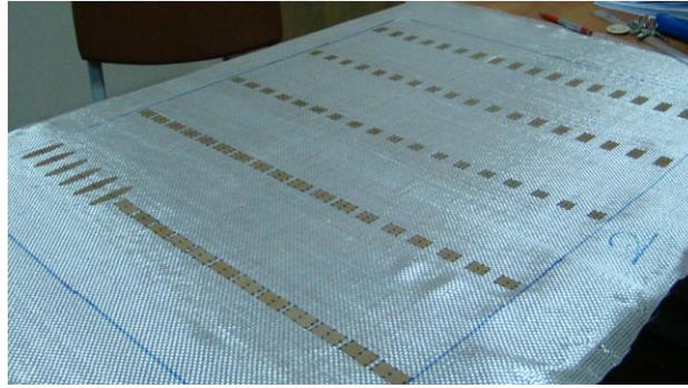
Figure 3.4 A layer which prepared to create delamination area
