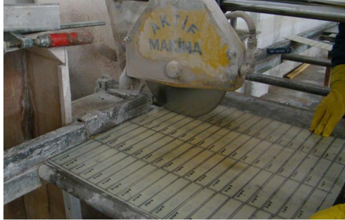
Figure 3.6 Cutting process of laminated composite plates
