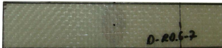
Figure 3.7 A specimen for lateral buckling test
