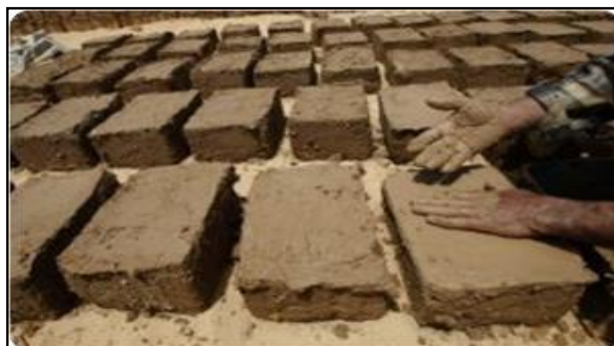
Figure 2.3 Production of adobe material [29]
