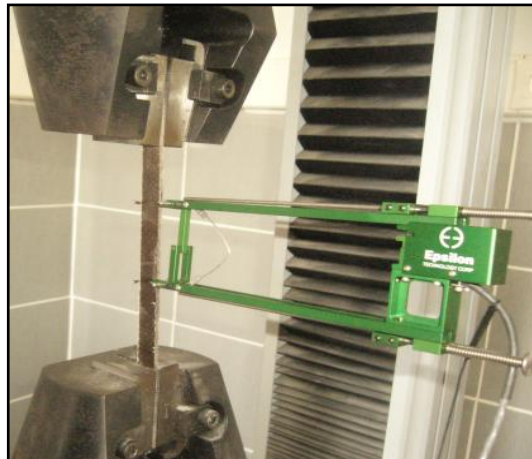
Figure 4.4 Typical single-axis extensometer, mounted on a tensile specimen.
