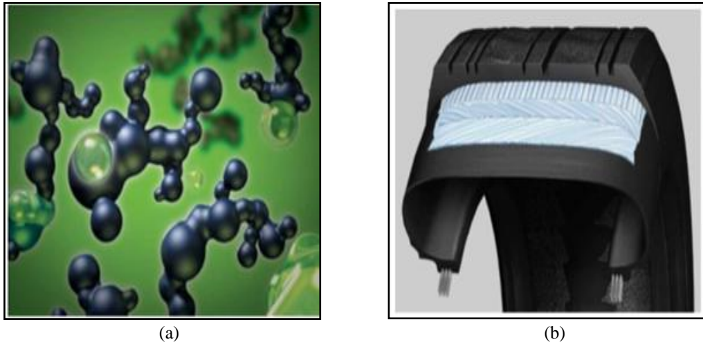
Figure 2.6 An image of (a) nano-composite and (b) the carbon black matrix materials in car tires [37]
