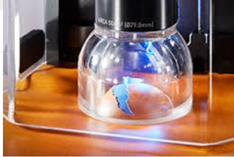
Şekil 2.13. Patlama mukavemet test cihazı ( www.james-heal.co.uk , 2016)
