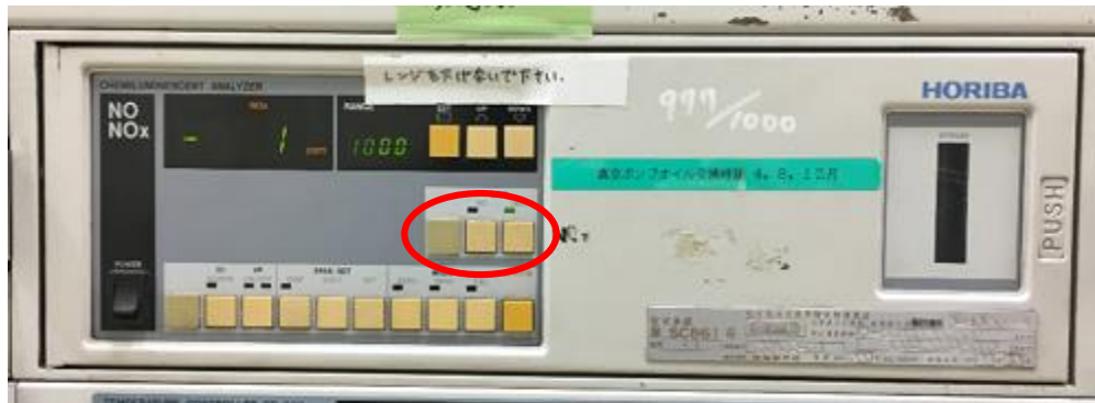
Figure 2.17. NO and NO x display unit
