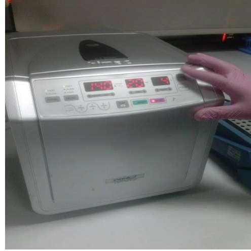
Resim 3. Santrifüj 14,000 rpm, 20 dk, +4 °C
