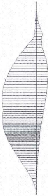
Envelope of Bending moments Extreme bending moment 324,30 kNm/m
